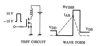
$$\begin{aligned} R_G &= 25 \ \Omega \\ V_{DD} &= 90 \ \text{V}, \ L = 17.4 \ \text{mH} \end{aligned} \quad E_{AS} = \frac{1}{2} \cdot L \cdot I^2 \cdot \left( \frac{B \text{VDSS}}{B \text{VDSS} - \text{VDD}} \right)$$
